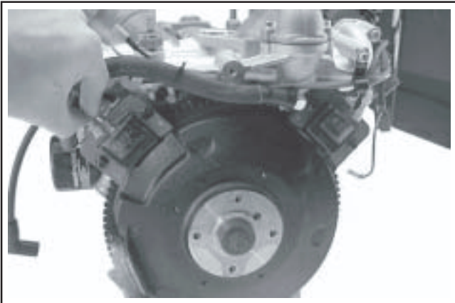
Figure 9-36. Removing Kill Leads from Ignition Modules.
