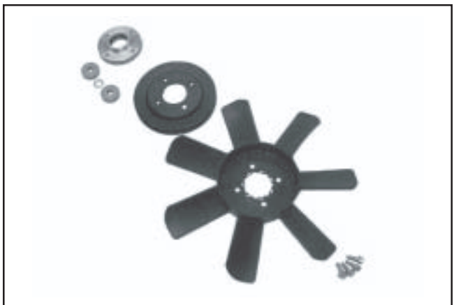
Figure 11-94. Fan Assembly Components - Disassembled Layout.
