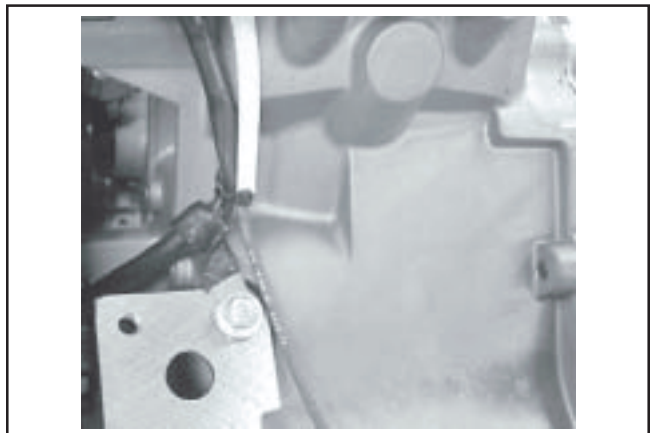
Figure 11-66. Side View of Stator and B+ Leads Tied to Clamp on Adapter.
