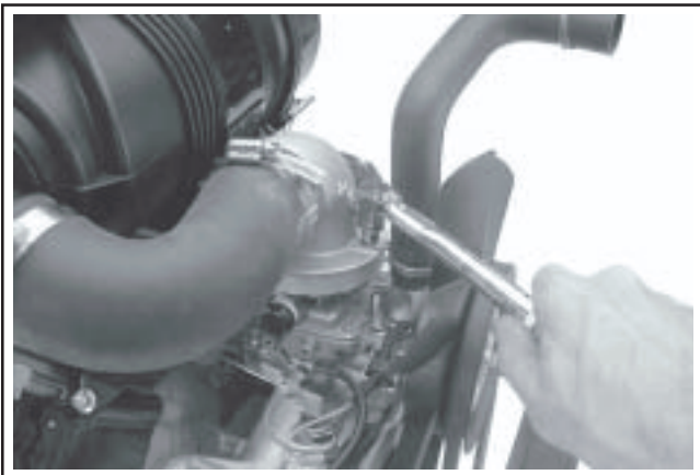
Figure 11-105. Torquing Elbow Mounting Screws.
