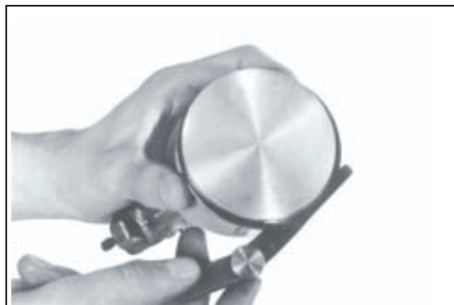
Figure 10-9. Measuring Piston Ring Side Clearance.
