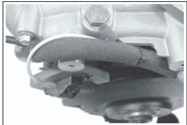
Figure 11-73. By-pass Hose and Wiring Routed within Cutout of Intake Manifold (some models).
