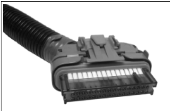
Figure 5B-19. “32 Pin” (MSE 1.1) Plastic-Cased ECU Connector.
