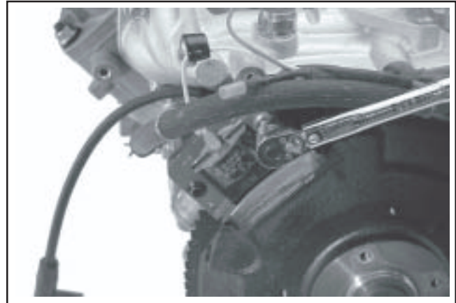
Figure 11-72. Torquing/Setting Ignition Module Gap.
