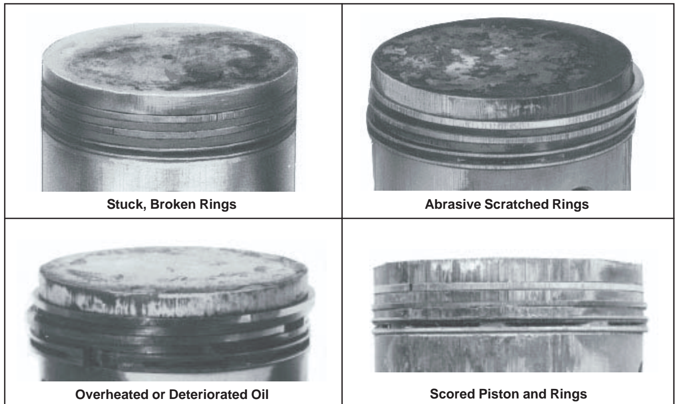
Figure 10-7. Common Types of Piston and Ring Damage.
