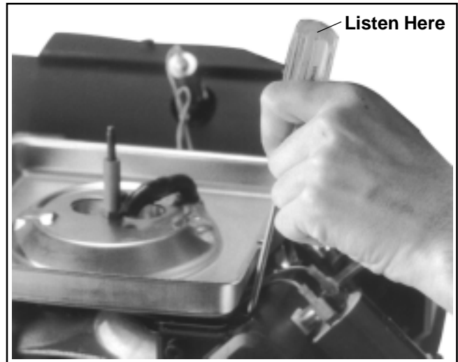
Figure 5B-15. Checking Injectors.
