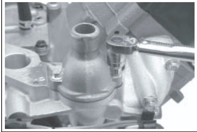
Figure 11-61. Torquing Thermostat Housing Screws.
