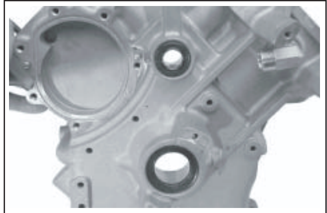
Figure 9-66. Oil Seals (Flywheel Side and Camshaft).
